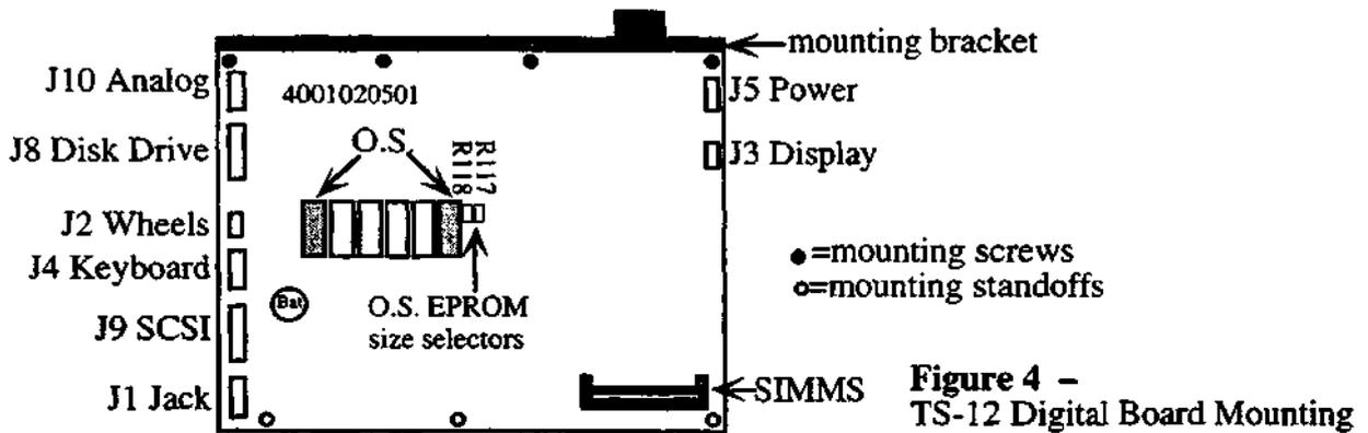
4. Pop the digital board off the three (3) standoffs holding the digital board to the I/O bracket by squeezing the standoffs with needlenose pliers, see **Figure 4**.
